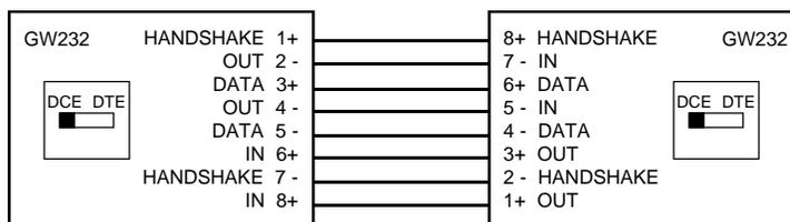
Diagram of two GW232 units connected in 8 wire Data and handshake configuration, extending the RS-232 interface. Full duplex serial channel with hardware handshaking.
