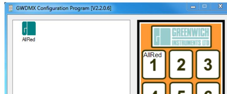
Once you are ready, you can connect the GWDMX to a spare USB socket, the software should automatically find the device and the “Transfer To GWDMX” button should be enabled. Click the transfer button and all of the sequences will be sent to the relevant button on the GWDMX.
