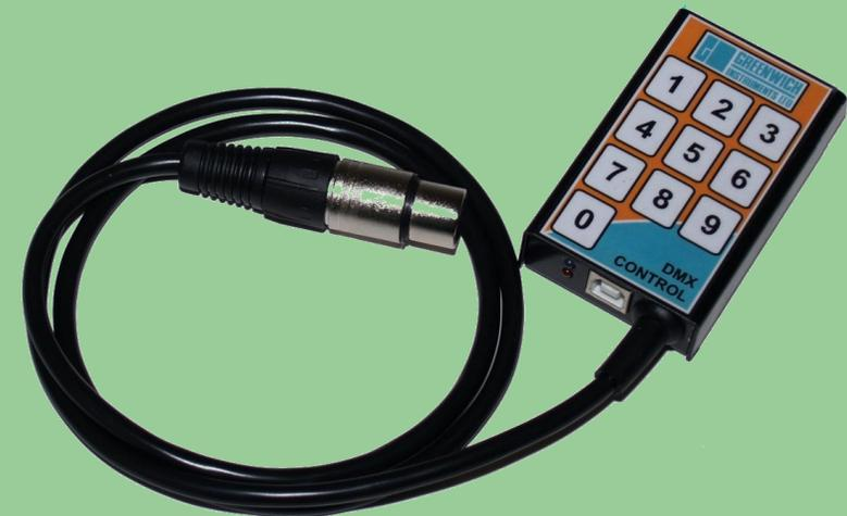
The GWDMX is a DMX-512 compatible lighting controller, designed for use by bands, DJ's, displays and remote applications. The GWDMX has ten programmable buttons, each button can hold a scene or a sequence of scenes, making it a really simple controller to configure and use. It's small size and low power requirements means it can run from a battery pack when a mains socket is not available.
